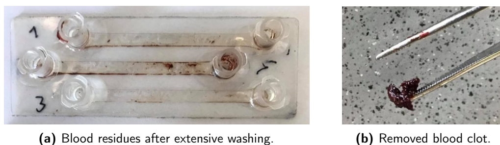
Figure 4.9: Effects of blood incubation with heparin-anticoagulated blood in microchannel chip.
