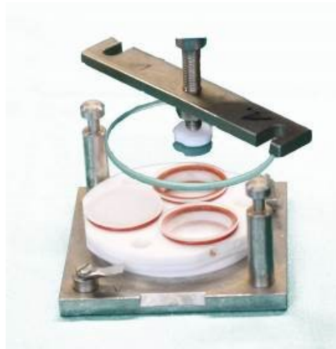
Figure 6.3: Blood incubation chamber for quasi-static hemocompatibility assessment.
