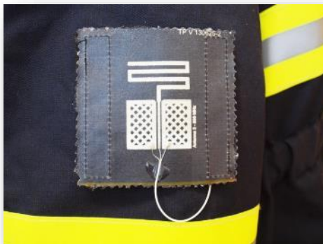
868 MHz antenna printed on textile substrate.
