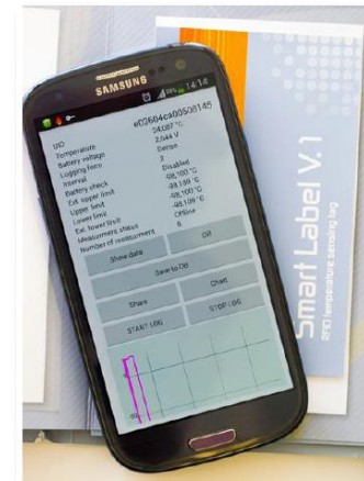
Smartphone application for label control and data transfer to cloud storage (NFC, Google Firebase)
