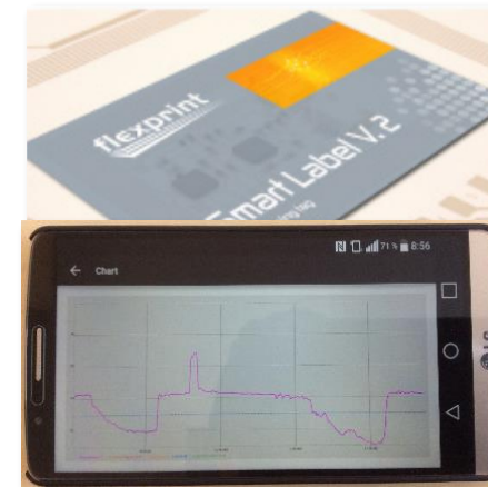
Smartphone application for label control and data transfer to cloud storage (NFC, Google Firebase)
