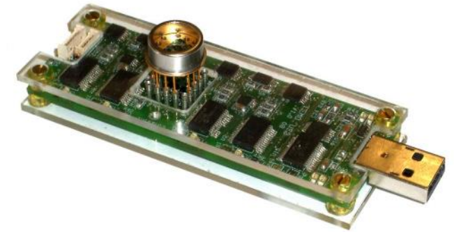
CNR-IMM 4-sensor MOX array readout electronics USB dongle (2007)
