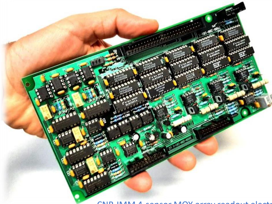
CNR-IMM 4-sensor MOX array readout electronics with proprietary digital communication interface (1999)
