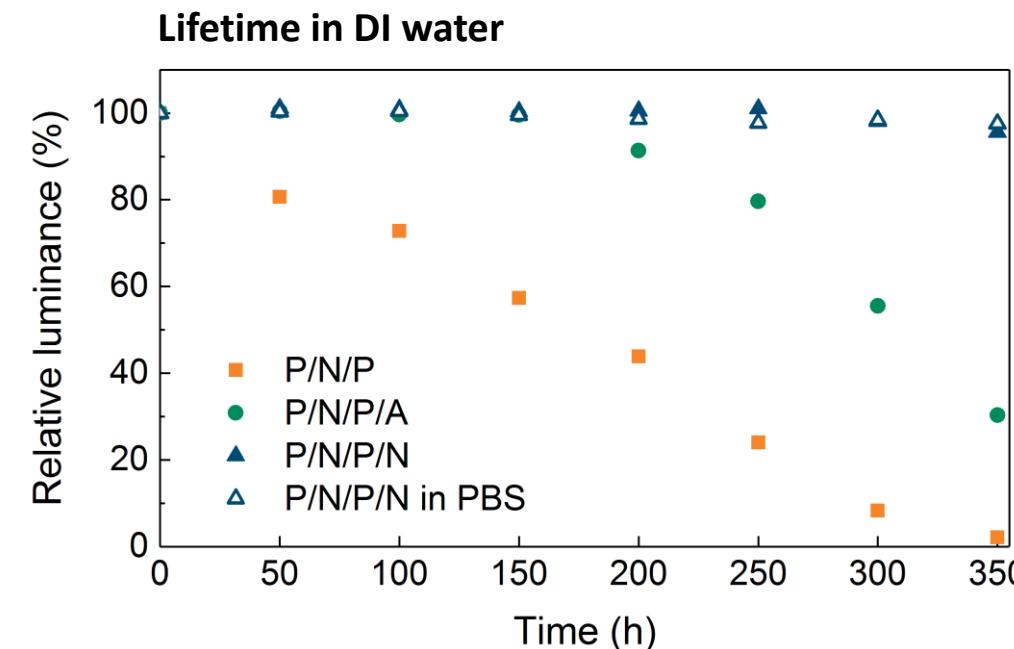
Encapsulation comprising parylene and ALD-processed  $\text{Al}_2\text{O}_3/\text{ZrO}_2$  layers
