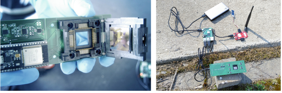
Fig. 7. Left: Nano-sensor array to detect Ammonia gas. Right: Wireless sensor node integrating an array of nano-sensors to detect Ammonia.
