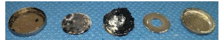
Destroyed coin cell because of a short circuit
