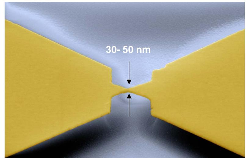
**Mechanically controlled break junction technique**
