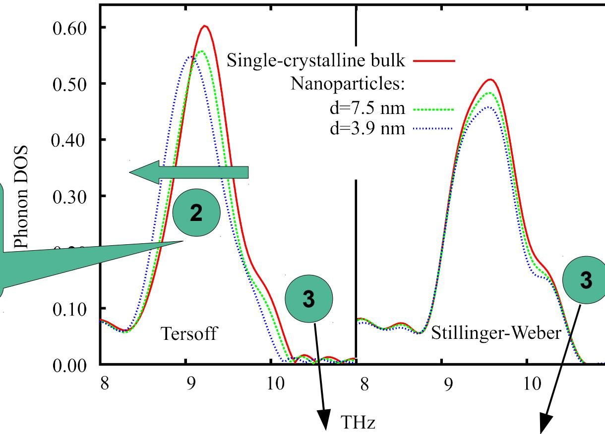
The shoulder at high frequency is shifted due to the confinement effect.
