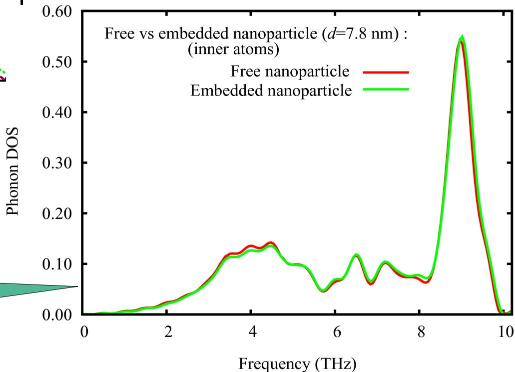
Vibrational modes of glassy matrix do not extend in the inner part of the embedded particle
