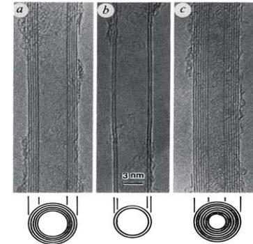
FIG. 1 Electron micrographs of microtubules of graphitic carbon. Parallel dark lines correspond to the (002) lattice images of graphite. A cross-section of each tube is illustrated. a. Tube consisting of five graphitic sheets, diameter 6.7 nm. b. Two-sheet tube, diameter 5.5 nm. c. Seven-sheet tube, diameter 6.5 nm, which has the smallest hollow diameter (2.2 nm).
