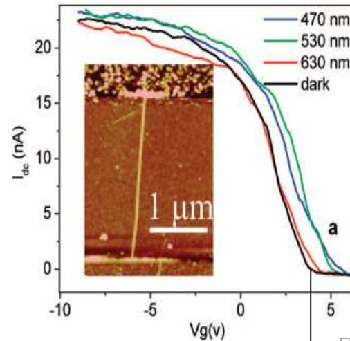
Threshold voltage shift of devices
