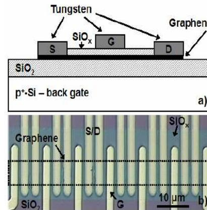
Non-volatile switching in graphene FED
