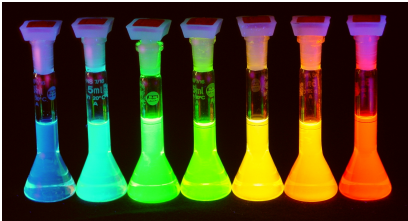
Fluorescence of Cadmium Selenide Quantum Dots
