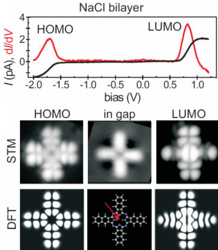
STP/STM of naphthalocyanine on 2MLNaCl/Cu(111)
