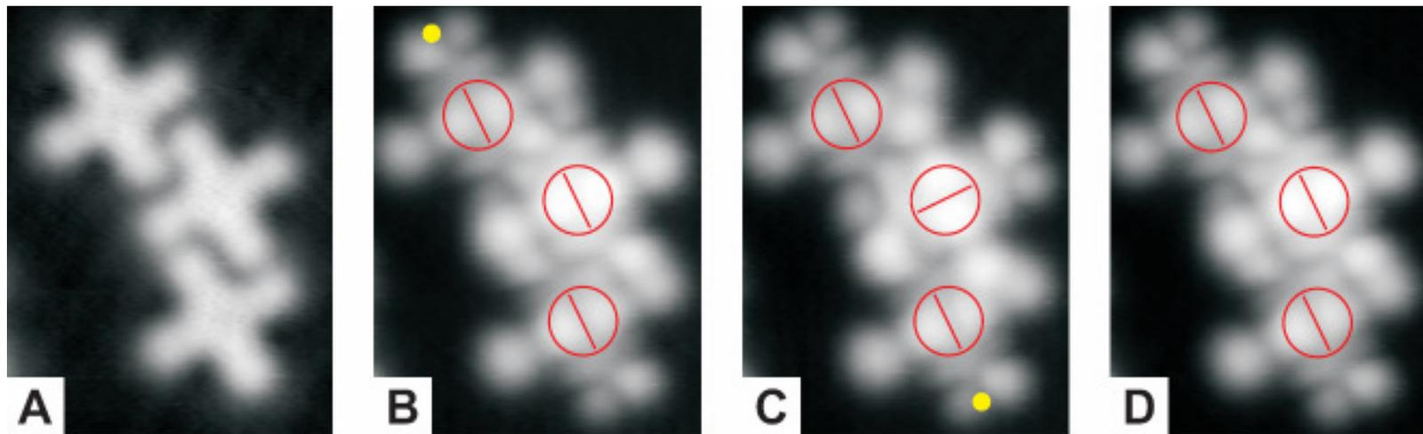
A: in gap image 0.3V. B-D Current injection through top/bottom molecules induces switching of middle one
