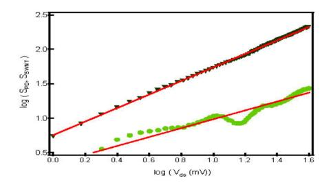
They implemented an AC modulation lock-in technique and designed a resonant tank-circuit (f = 15 Mhz) together with a home-built cryogenic low-noise preamplifier 2.2nV/ sqrt (Hz). **The measurements were performed at 4 kelvin**
