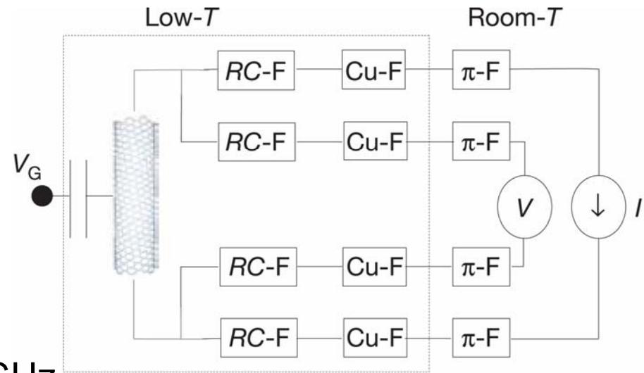
for the 2-stage RC-filter they claim to see a damping of 40 dB per decade instead of the 20 dB for usual systems
