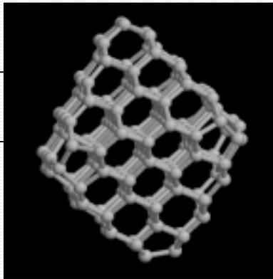
Diamond structure is stabilized by electron charging
