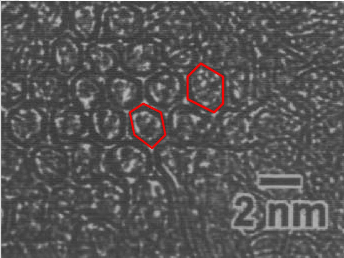
TEM image of a lattice of polygonized tubes
