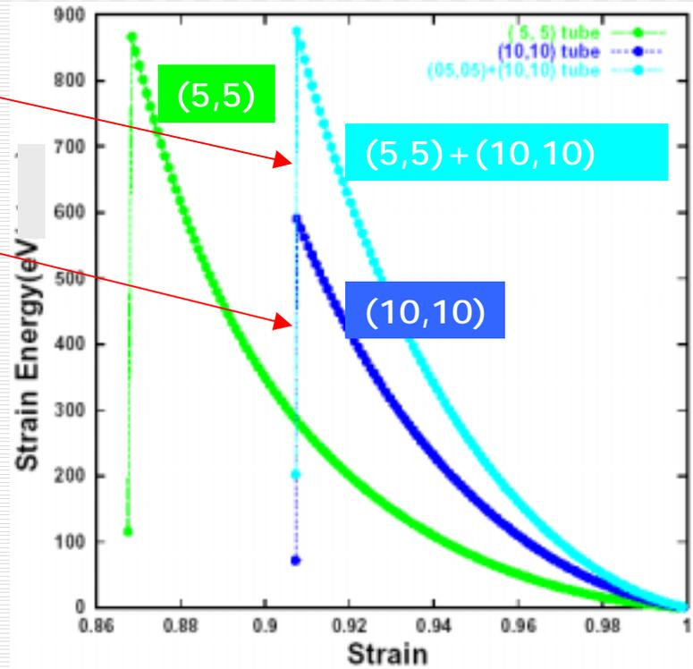
○ Buckling point of DWcnt is determined at outer CNT.
