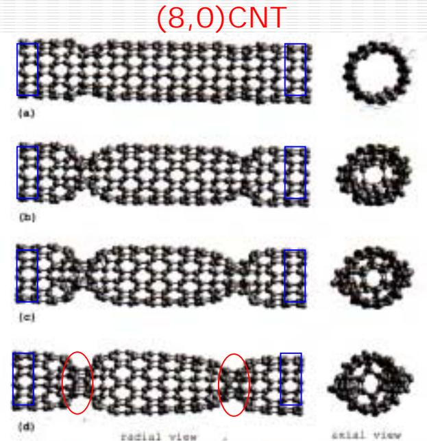
FIG. 2. Four stages of spontaneous plastic collapse of the 12% compressed (8,0) carbon nanotube showing: (a) nucleation of the deformations; [(b) and (c)] inward collapse at the locations of deformations; and (d) graphitic to diamondlike structural transition at the location of the collapse.
