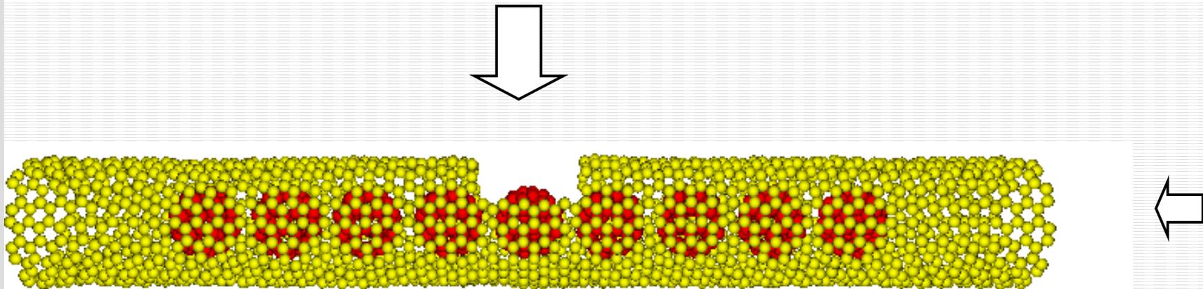
⇒ After 15 ps at room temperature, the encapsulation of fullerenes remain inside .
