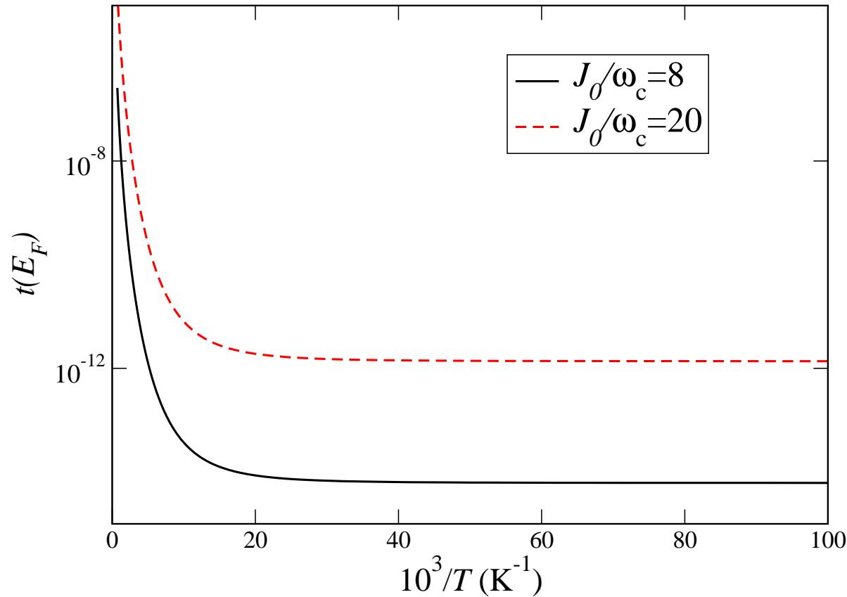
Activated behaviour:  $t(E_F) \sim e^{-\text{const.}/k_B T}$
