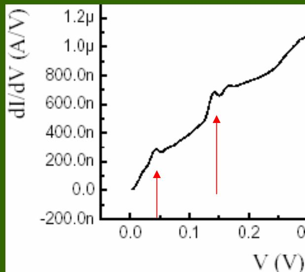
Inelastic electron tunneling spectra of C8 dithiol SAM obtained from lock-in second harmonic measurements with an AC modulation of 8.7 mV (RMS value) at a frequency of 503 Hz ( $T = 4.2$  K). Peaks labeled \* are most probably background due to the encasing Si<sub>3</sub>N<sub>4</sub>
