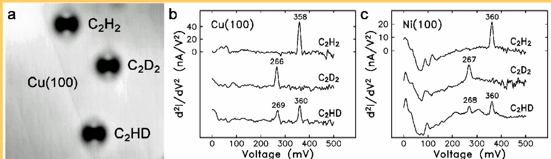
STM image (a) and single-molecule vibrational spectra (b) of three acetylene isotopes on Cu(100) at 8 K. The vibrational spectra on Ni(100) are shown in (c). The imaged area in (a), 56 Å × 56 Å, was scanned at 50 mV sample bias and 1 nA tunneling current
