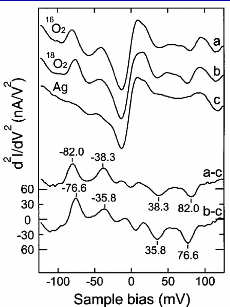
**Single molecule vibrational spectra obtained by STM-IETS for  $^{16}\text{O}_2$  (curve a),  $^{18}\text{O}_2$  (curve b), and the clean Ag(110)surface (curve c). The O<sub>2</sub> spectra were taken over a position 1.6 Å from the molecular center along the [001] axis.**
