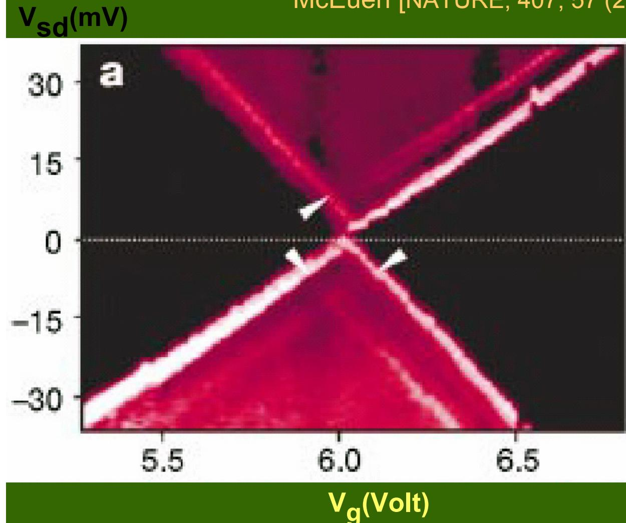
Two-dimensional differential conductance ( $\partial I / \partial V$ ) plots as a function of the bias voltage (V) and the gate voltage ( $V_g$ ). The dark triangular regions correspond to the conductance gap, and the bright lines represent peaks in the differential conductance.
