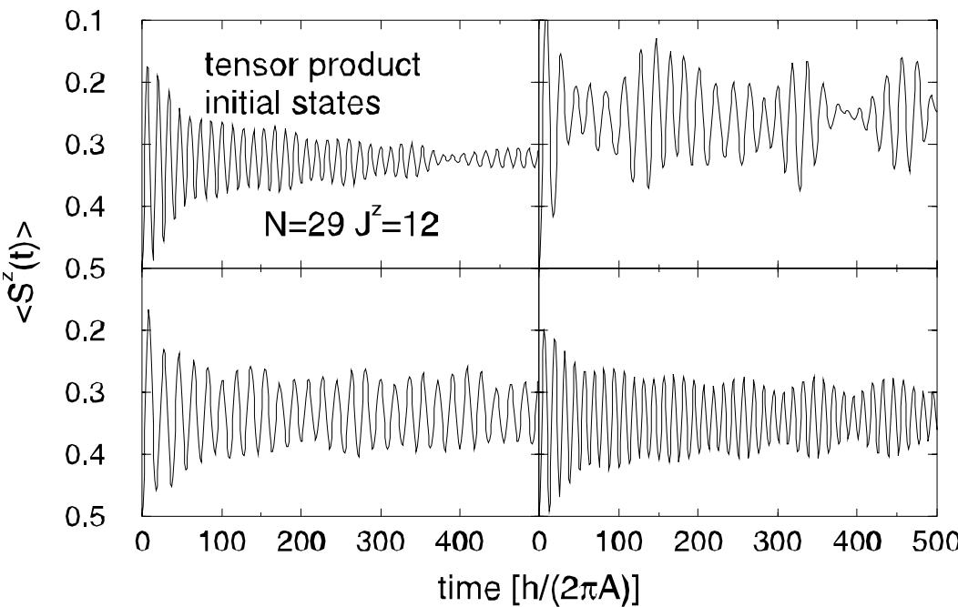
Electron spin dynamics for an initially randomly correlated nuclear spin system. The electron spin dynamics is practically independent of the realization of the random initial nuclear state.
