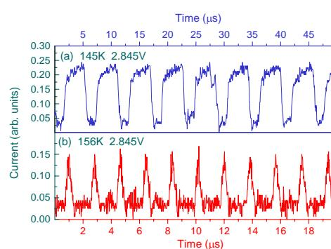
self-sustained current oscillation in superlattice caused by NDR
